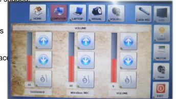
will display both the visual and audio outputs from the selection. When computer or Laptop are selected, the volume settings will remain below to control the Gooseneck Microphone, Wireless Microphone and main volume levels.
